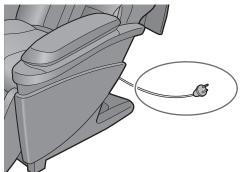
Be sure to push the connector all the way into the appliance inlet.
